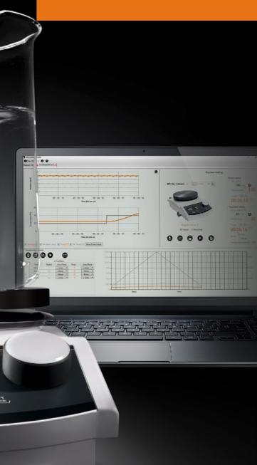
programming of ramps and interval processes. With RS 232 interface for detailed process documentation directly on the PC.
